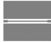
(a)信号线和测量触点宽度不同的短波导 (a)Short CPW (pad is thicker than signal line)
