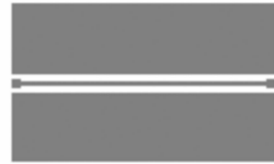
(b)信号线和测量触点宽度不同的长波导 (b)Long CPW (pad is thicker than signal line)
