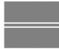
(c)信号线和测量触点宽度相同的短波导 (c)Short CPW (pad is as thick as signal line)
